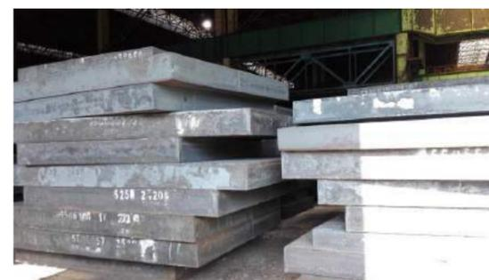
ASTM A588Grade K(A588GRK) Weather Resistant Steel Plate
